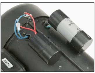
Figure 74. Capacitor wiring.
